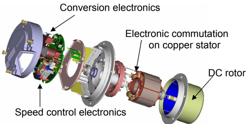
In the development of electronics to convert alternating current supply to direct current supply, many other features were made available. The two main features being:
