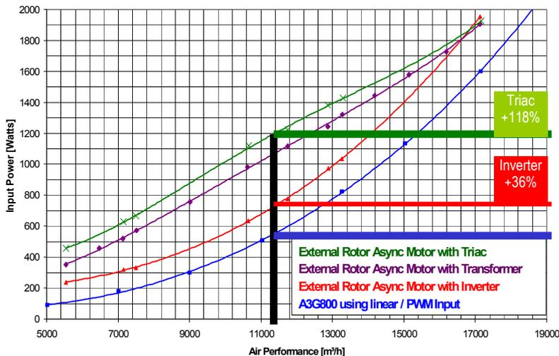
As can be seen, EC technology approached the theoretical third power relations set out by the fan laws and all other speed control techniques have inherent losses in their methodology. For instance at the same duty point inverter control techniques can typically absorb 36% more power than EC and similarly triac control systems consume 118% more.
