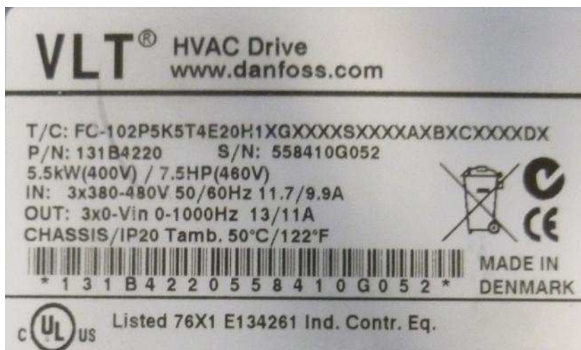
Figure 11: Type plate of the frequency inverter utilised with the PM motor in standard motor shape
