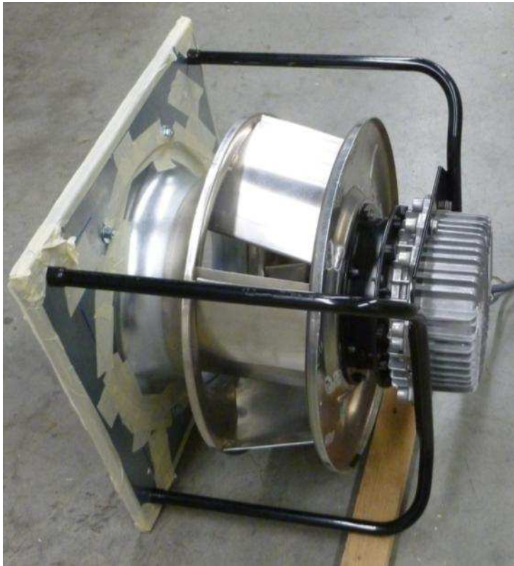
Figure 6: Picture of sample 1 - centrifugal fan with EC motor
