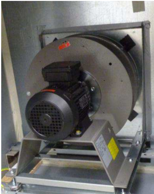
Figure 8: Picture of sample 2 - centrifugal fan with PM motor with standard motor shape
