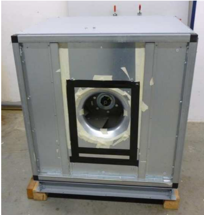
Figure 4: HVAC unit casing (ALKO) viewed to outflow
