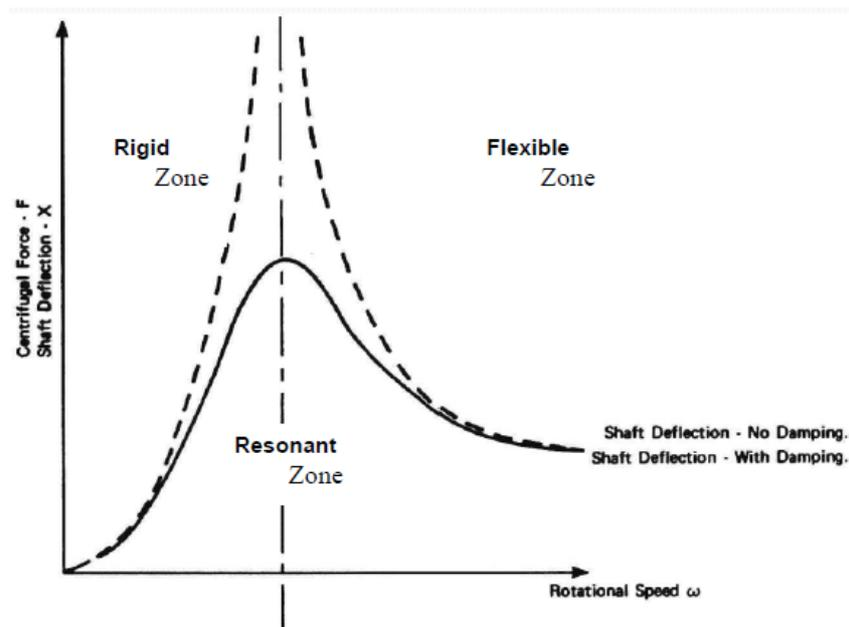
Figure 1: Rigid, flexible & resonant zones, *Fundamentals of Vibration Measurement and Analysis Explained*. Source: [www.Lifetime-reliability.com](http://www.Lifetime-reliability.com), 25 October 2016.
