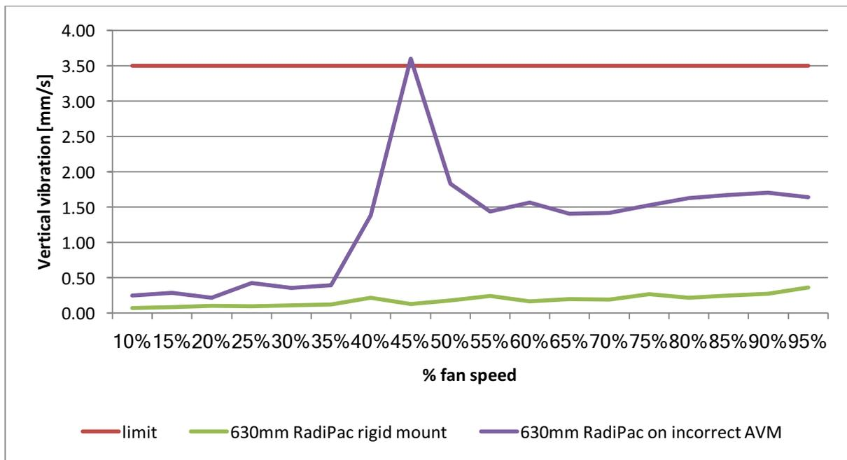
Figure 3: Radial vibration vs fan speed, as measured on site installed in application, before and after removal of AVM.
