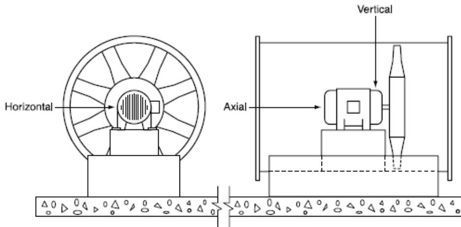
Figure 2: Axial, vertical and horizontal vibration measurement points, ANSI/AMCA Standard 204-05 Balance Quality and Vibration Levels for Fans, 21 October 2016.
